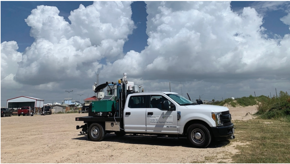
Researchers at Brookhaven's Center for Multiscale Applied Sensing integrated a suite of weather instruments on a truck to create a mobile observatory capable of measuring climate data while driving through local neighborhoods. [Courtesy Brookhaven National Laboratory]
