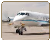
The Atmospheric Radiation Measurement (ARM) user facility employs this G-1 aircraft to measure a range of aerosol and cloud properties, as well as collect gas-phase measurements. [Courtesy U.S. Department of Energy Atmospheric Radiation Measurement (ARM) user facility.]
