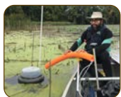
A researcher in a canoe uses a floating chamber and a gas analyzer to measure methane emission from Old Woman Creek wetland in Ohio. [Courtesy The Ohio State University]
