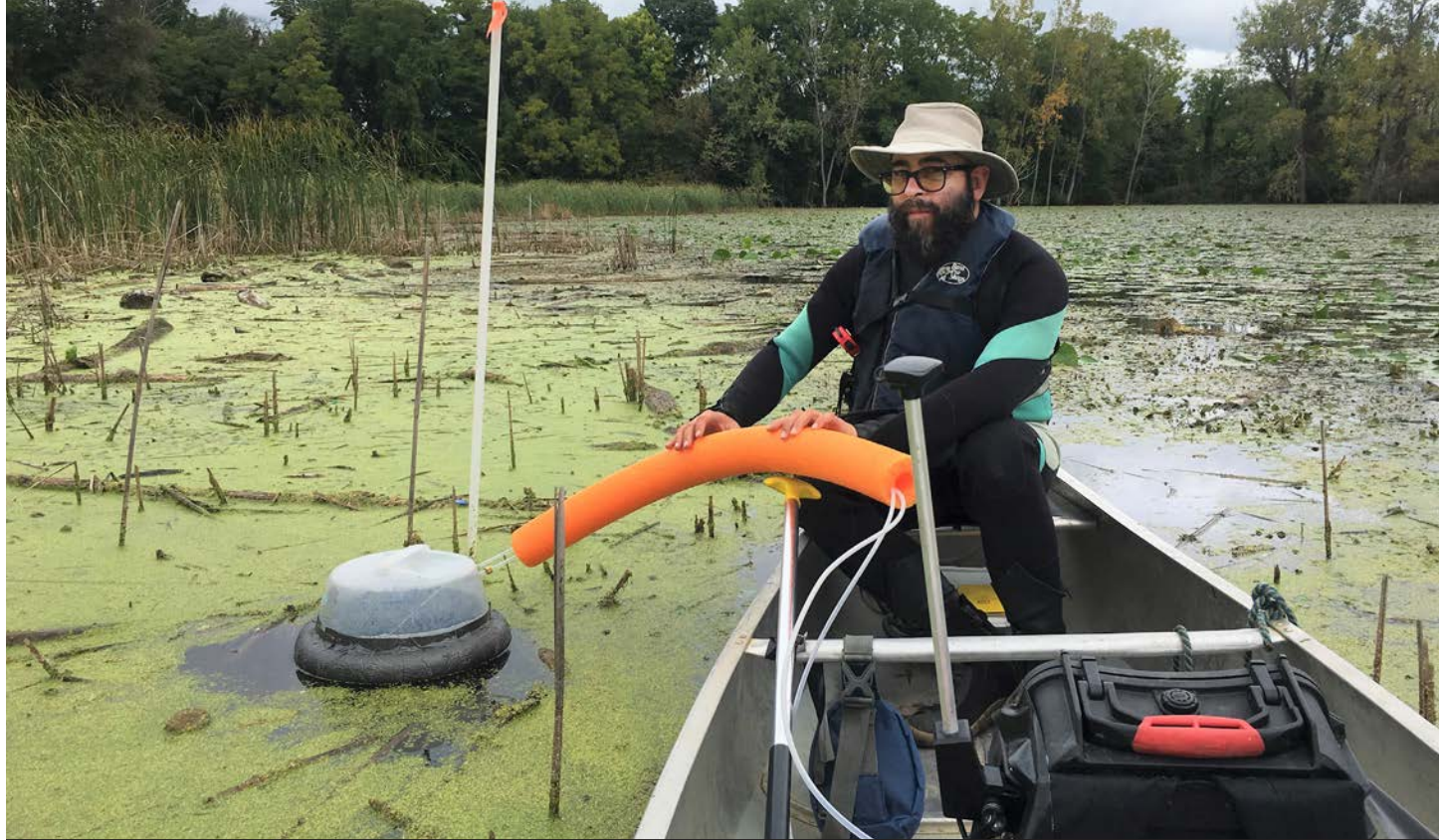
A researcher uses a floating chamber and a gas analyzer to measure methane at Old Woman Creek. [Courtesy The Ohio State University]
