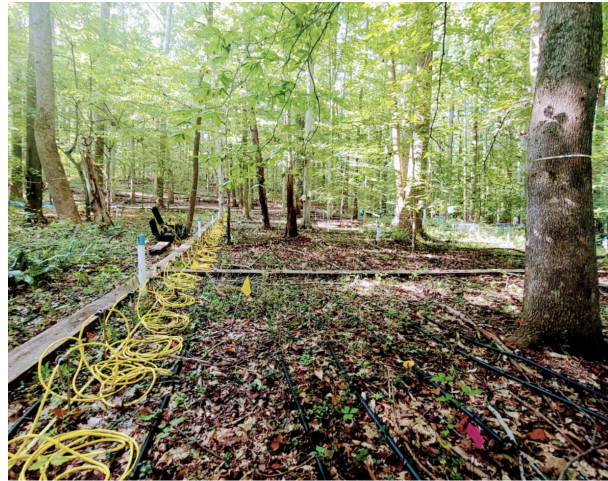
Fig. 2.2. Terrestrial Ecosystem Manipulation To Probe the Effects of Storm Treatments. TEMPEST is a decade-scale experiment designed to test the effects of seawater and freshwater flooding on ecosystem state and function. Throughout the year, over 1.4 million observations are captured every month, spanning weather conditions, vegetation dynamics, soil conditions, and groundwater and open water chemistry. During the treatment events, soil and water sampling and soil and plant trace gas measurements are manually conducted. [Courtesy Nick Ward, Pacific Northwest National Laboratory]
