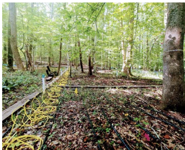
Fig. 2.2. Terrestrial Ecosystem Manipulation To Probe the Effects of Storm Treatments. TEMPEST is a decade-scale experiment designed to test the effects of seawater and freshwater flooding on ecosystem state and function. Throughout the year, over 1.4 million observations are captured every month, spanning weather conditions, vegetation dynamics, soil conditions, and groundwater and open water chemistry. During the treatment events, soil and water sampling and soil and plant trace gas measurements are manually conducted. [Courtesy Nick Ward, Pacific Northwest National Laboratory]
